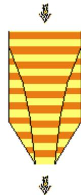
It is clear from this that the silo under investigation is subject to funnel flow. That is, the centre column of material flows out of the silo and slowly draws the outer edges into the funnel. At certain points the material at the edge will become unstable and there will be a slide of this material. This explains the sudden increases in the levels shown by the wire guided radar and the ultrasonic. This is further supported by the return to similar traces while filling.
