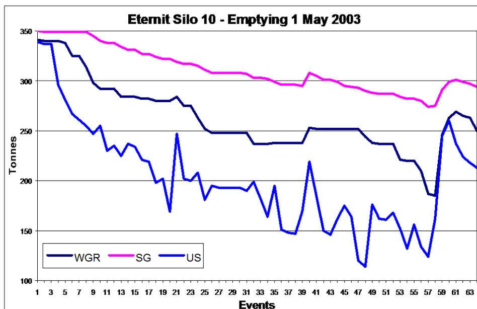
From this graph it can be seen that at the start there is a step change between the Strain Gauge system and both the Wire Guided Radar and the Ultrasonic. This is evidence of a certain
