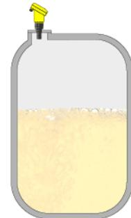
Latest microprocessor technology and proven software select the level echo from a number of false reflections and measure it exactly.
