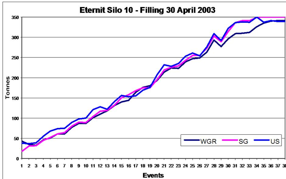
The recording of the filling process showed that the systems report relatively accurately compared to each other while the silo is being filled. The next part of the process was to monitor the emptying cycle from the full point to a lower level. This was completed the next day when Eternit put the silo back into production.
